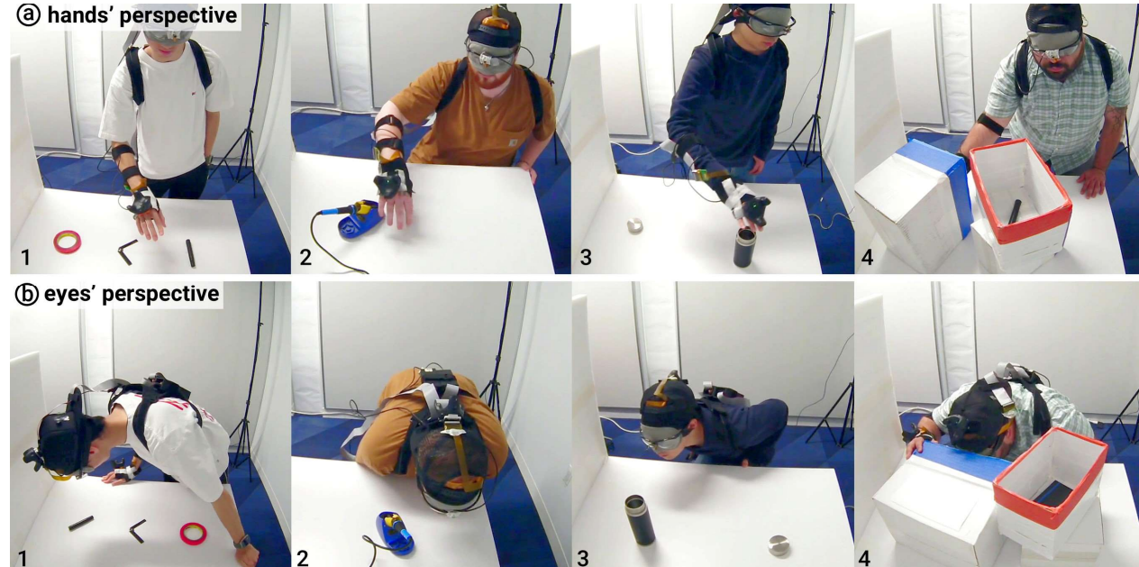
Figure 5: (a) When using the hand-device , participants explored the objects by scanning with their hand. (b) The eye-device led to unergonomic behaviors such as crouching and craning necks. (Photos with consent from participants)
